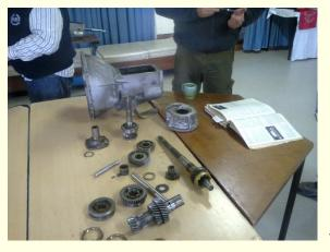
5. Wear on the clutch actuation shaft bushes should also be measured in the bushes replaced if there is excessive movement.
